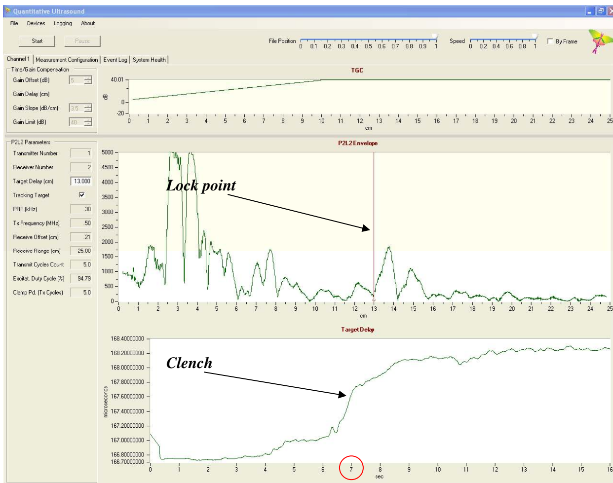
Figure 4 Locking on back surface reflection
