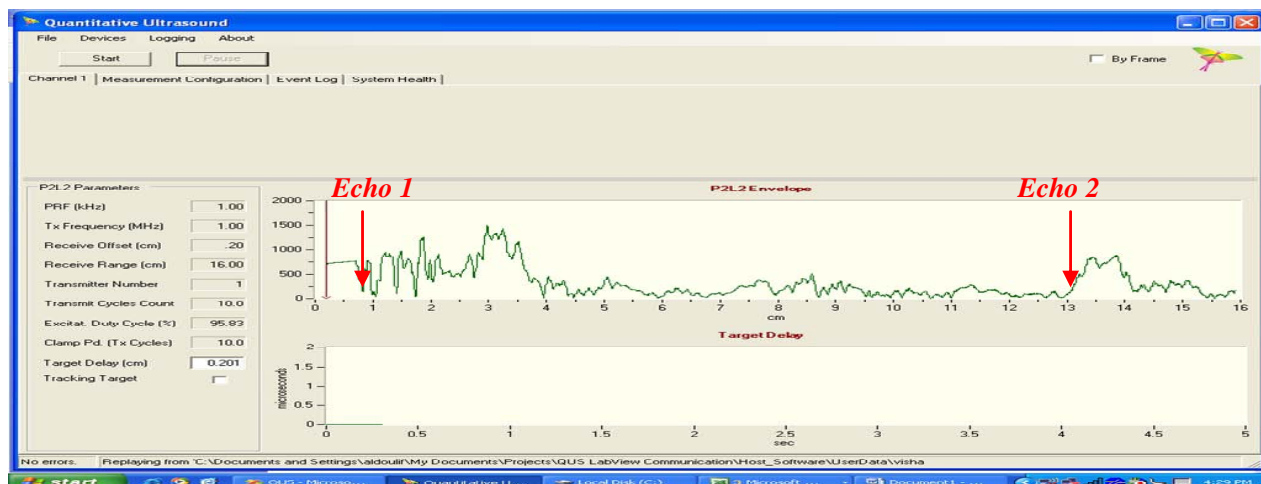
Figure 3 Echoes tracked for the jaw clenching tests using PPLL software.
